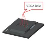
Step 5: Attach the LCD display to the wall, and follow the instructions in the wall-mounting kit.
